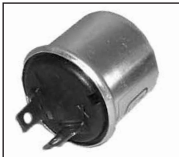
Chalk's Part #: 552 12V Round, Variable Load, Flashes Up To 6 - 32 CP Bulbs For Hazard Warning, 2 Blade
