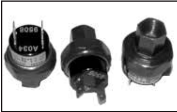
Chalk's Part #: 29-30104 Low Pressure Switch, 2 Blades, Normal Open, On 30 PSI / Off 5 PSI
