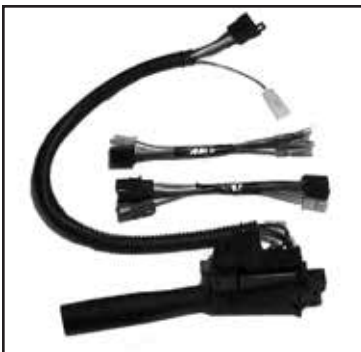
Chalk's Part #: 1697207C91 Turn Signal Switch, "S" & 3000 Series, Without Dimmer Switch 3566941C91 Use Conversion Plug # 2032852C92
