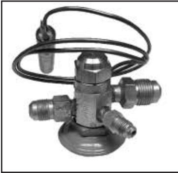
Chalk's Part #: 31-10979 - Expansion Valve 3 Ton R134A, 26" External Equalizer, In - 3/8" Out - 1/2"
