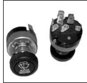
Chalk's Part #: W405 Push In Washer, Windshield Wiper Switch, 5 Blade W410K - Knob
