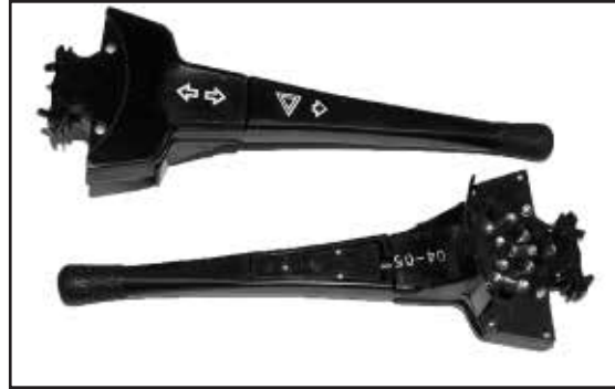
Chalk's Part #: 471302C94 Old style Turn Signal Switch. The New Style #s 1697207C91 , and 2002875C91 Are Available And In Stock.
