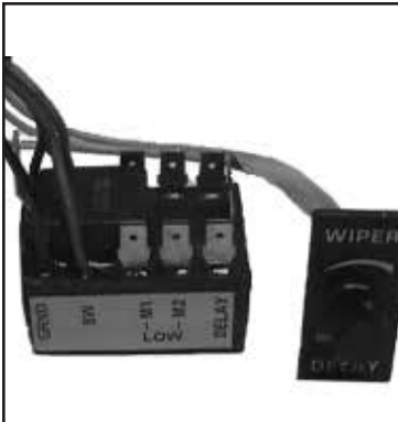
Chalk's Part #: W412 Wiper Modul (Thomas) Switch And Module, 8 Blade
