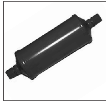
Chalk's Part #: 37-10860 Filter Drier, 1/2" x 1/2" FO, 30 Cu. In., 3" Dia, Drier, 10" Long
