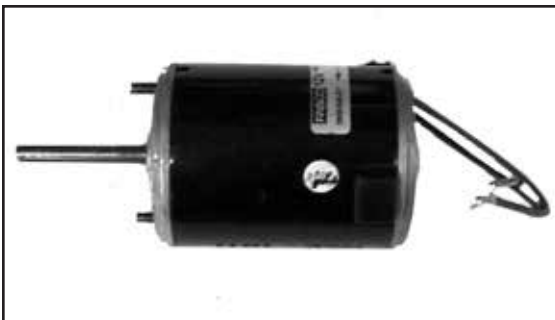
Chalk's Part #: HM-350 Heater Motor, AmTran,, 5/16" Single Shaft CCW , Single Speed, 12V
