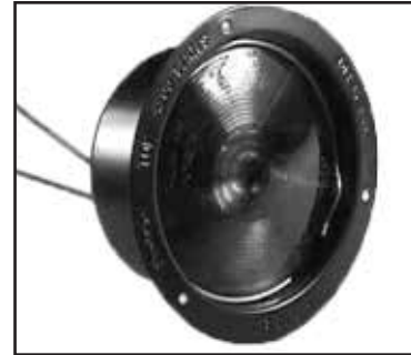
Chalk's Part #: 50232 DOUBLE CONTACT , 2 Wire Pigtail . Heavy Duty Steel, Recessed Construction With Baked Black Enamel Finish, Lens Held By Snap-Ring For Easy Bulb Change. Grote Bulb: # 1157 Lens: # 90012 (Red)
