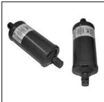
Chalk's Part #: 37-10866 Drier, Trans Air, 1/2" x 1/2" MFL, 30 Cu. In., 3" Dia
