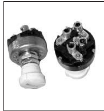
Chalk's Part #: CSB-405 Universal Wiper Switch W/Wash Feature, 4 Plug Ins
