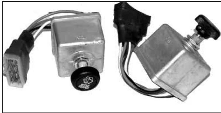
Chalk's Part #: W408 Wiper Switch Controls Two Motors 12VDC, For Motors Without Dynamic Parking Including United Technologies And Sprague Devices Motors, Blue Bird 8 Way Female Connector With Knob, Push To Wash
