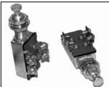
Chalk's Part #: S147 Door Switch, Normally On, OFF When Plunger Depressed 4 Screw S154 - Same w/ Blades
