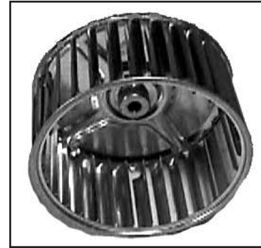
Chalk's Part #: 1567270 Blower Wheel, CCW , 2 7/8"H x 5 1/4" D, Steel
