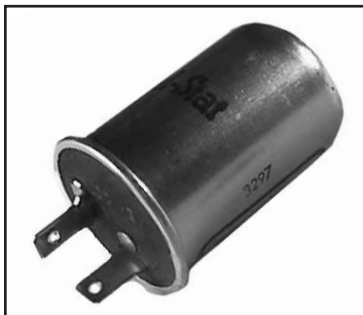
Chalk's Part #: 536 12V Round, Heavy-Duty, Variable Load, Flashes Up To 6 - 32 CP Bulbs For Hazard Warning, 2 Blade
