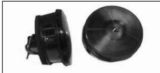
Chalk's Part #: 2500 DOUBLE CONTACT , Narrow Stop/Tail/Turn Light W/ License Illuminator, Dual Cont., Plastic Housing, Entire Lamp Extends Less Than 2" From Mounting Surface. 2 Wire, Mounts On 2" Centers Snap On Lens, Weldon Bulb #: 1157 Lens #: OC11-1308-00 - Red Snap Lock
