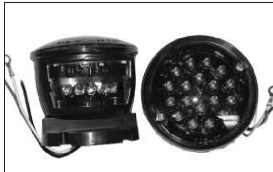
Chalk's Part #: 9154 LED 4" Red S/T/T (18 Diodes) W/License Light (5 Diodes), Doran
