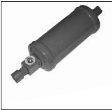
Chalk's Part #: 37-10886 Rifled Air Drier With Sight Glass 30 Cu In 1/2" MIO x 1/2" MIO, 3" Dia, 10" OA
