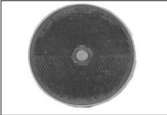
Chalk's Part #: 57A & R 3" Center Mount, Plastic Housing Lens, Hermetically Sealed Molded Insert For Center Mount Screw, Prevents Cracking, Reflector, Available In Amber & Red
