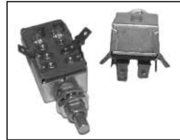
Chalk's Part #: S119 MOMENTARY Door Switch, Same As S101 Except For Blade Terminal Normally ON, OFF When Depressed, 6 Blade
