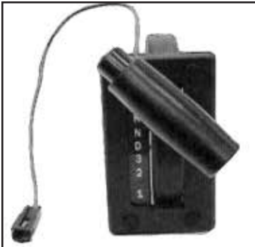
Chalk's Part #: 2006987C91 Shifter Control For Allison Trans. AT545 1693574C91 "T" Only
