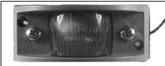
Chalk's Part #: 122A & R Armored, Plastic Housing, Pass-Through Mounting Holes For Installation W/O Disassembly, Flat Back Eliminates Need For Socket Holes, Clearance Marker Light; 3 1/8" (Center Mounting), Peterson Bulb: # 193 or # 194 (Rough Life) Lens: # 124-15A Amber Lens: # 124-15R Red
