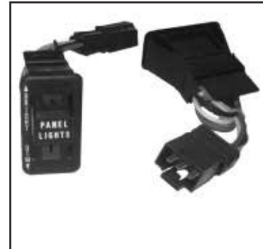
Chalk's Part #: R439 AMTRAN Control Panel Lights, Rheostat Type, 3 Wire R439-1 - 5 Wire B-bird
