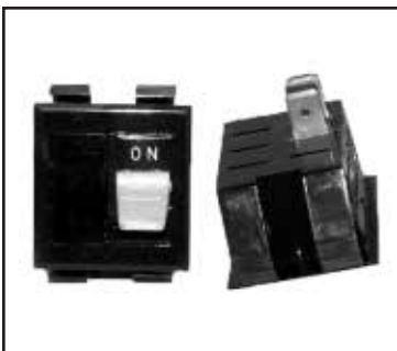
Chalk's Part #: T834 1 Position One Side Blank One Side OFF-MOMENTARY ON, Snap In Mount, 2 Blade
