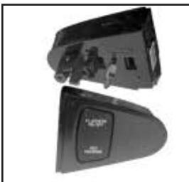
CTP #: CSB-7012 Switch Flasher On/Off In Steering Wheel, IH
