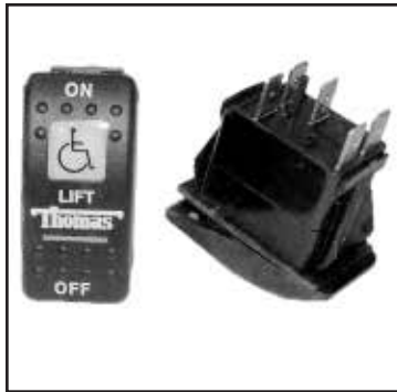
Chalk's Part #: R418 THOMAS Rocker, Lift, ON-OFF, W/Red Pilot Light, 5 Blade
