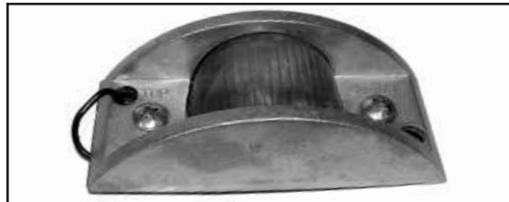
Chalk's Part #: 124A & R Clearance Marker Light, Cast Metal Housing, Pass-Through Mounting Holes Permit Installation W/O Disassembly. Flat Back Eliminates Need For A Socket Hole, 3 1/8" (Center Mounting), Peterson Bulb: # 193 or # 194 (Rough Life) Lens: # 124-15A Amber Lens: # 124-15R Red
