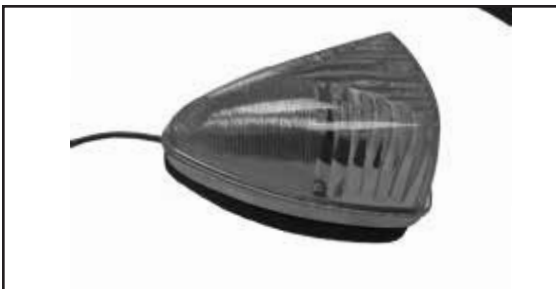
Chalk's Part #: 150A & R Cats Eye, (Remove Lens To Mount) 2 Screws To Mount Base, KD Bulb: # 168 Blade Type Or # 193 Lens: # 8861A Amber # 8861 Red Shield: # 5052S
