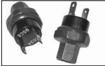
Chalk's Part #: 29-30120 High Pressure Switch , On 330 PSI Normal Closed, Off 230 PSI
