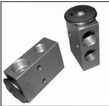
Chalk's Part #: 31-30927 Expansion Block Liq In 3/8" Out 1/2" Suc In 5/8" Out 5/8", 2 Ton R134a
