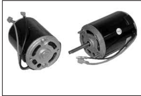
Chalk's Part #: HM-330 Heater Motor, Thomas, AmTran 5/16" Shaft, 1 1/2" Shaft Length Clockwise / Counter Clockwise , Single Speed, 12V
