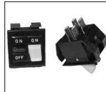
Chalk's Part #: T833 2 Position Split, White Side OFF-MOMENTARY ON Black Side ON-OFF, 4 Blade
