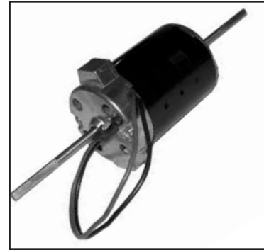
Chalk's Part #: 26-14522 Blower Motor, Double Shaft, Rev, For 26-19912 12V , 1 Speed, Blower Assembly, 3" Dia., Shaft Length 4"
