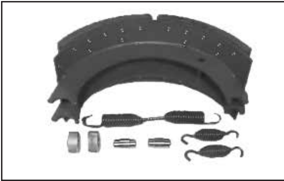
Eaton GH4311EJ 16 1/2" X 7", Rear Use Brake Kit # CQ67319 Return Spring O/A 10 7/8" X 1 1/8"
