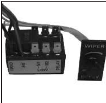
Chalk's Part #: W412 Wiper Module (Thomas) Switch and Module, 8 blade
