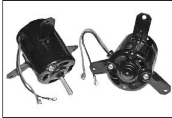
Chalk's Part #: HM-347 Heater Motor, Wayne Body With 3 Brackets, 5/16" Shaft Size, CW/CCW , 1 Speed, 12V SEE HM-360
