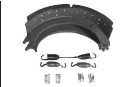
Spicer GD4709ES2J Extended Service, Eaton 16 1/2" X 7", Rear Use Brake Kit # CQ65481
